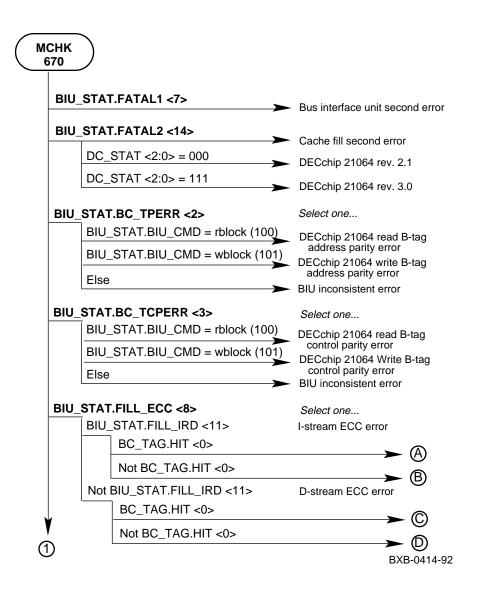
Figure 14-5 Processor Machine Check 670 Parse Tree (Continued)
