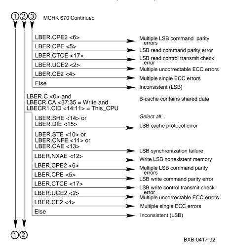
Figure 14-5 Processor Machine Check 670 Parse Tree (Continued)
