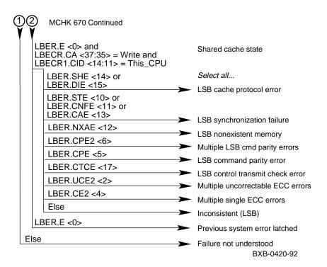
Figure 14-5 Processor Machine Check 670 Parse Tree (Continued)
