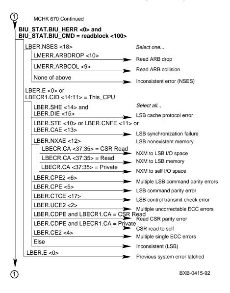
Figure 14-5 Processor Machine Check 670 Parse Tree (Continued)
