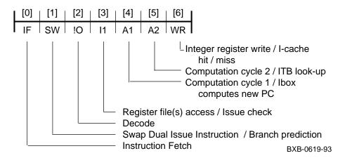
Figure 4-3 Memory Reference Pipeline
