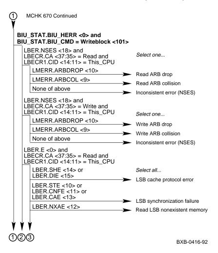
Figure 14-5 Processor Machine Check 670 Parse Tree (Continued)
