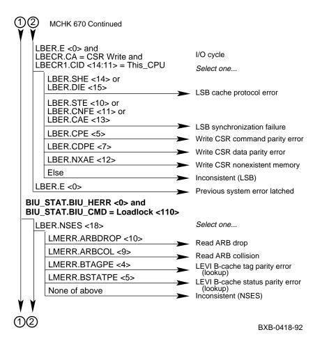
Figure 14-5 Processor Machine Check 670 Parse Tree (Continued)
