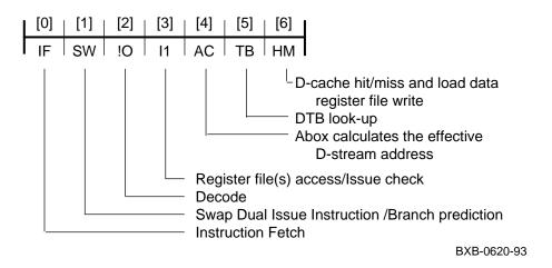
Figure 4-4 Floating-Point Operate Pipeline
