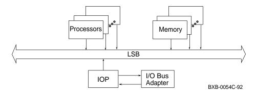
The CPU module is an Alpha AXP architecture implementation that runs optimized versions of OpenVMS AXP and DEC OSF/1 AXP. It operates in multiple as well as single processor configurations.
