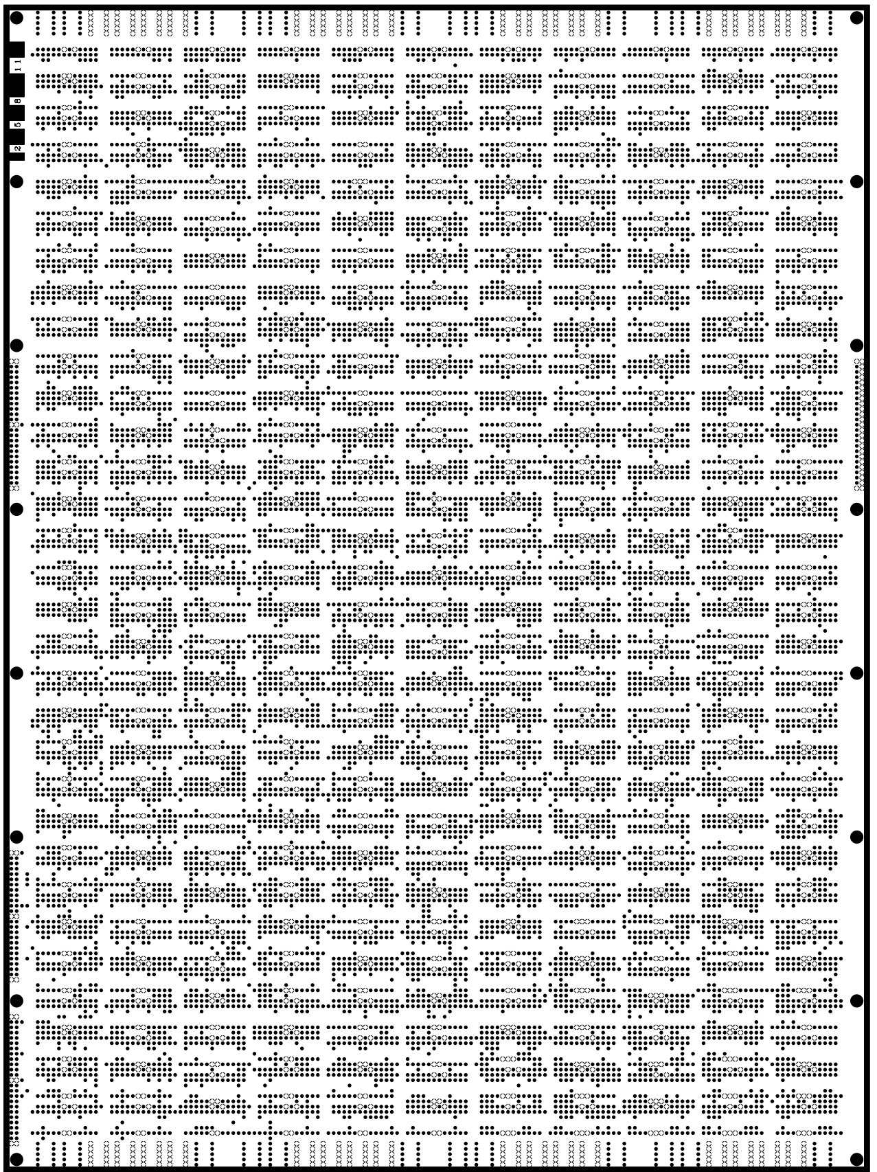
Figure 22: Titan Coprocessor Ground Plane
