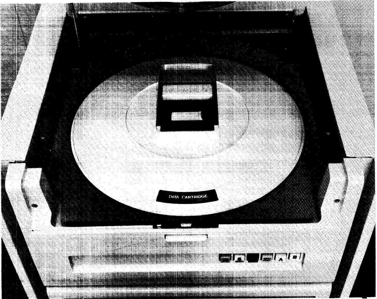
Figure 6-7 Cartridge Locked in Shroud
