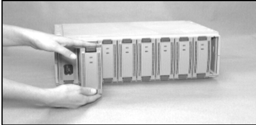
Figure 1–3 Removing an SBB from the Shelf
