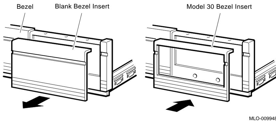
2. From inside the enclosure, push out the blank bezel insert that covers the right storage slot on the lower drive-mounting shelf.
