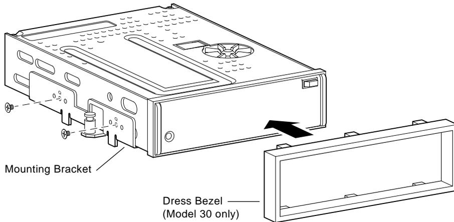
**Figure TZKxx-3 Installing the Bezel Insert**
