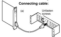
Attach the 50-way loopback connector (male) to the port or cable to be tested.
