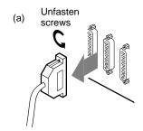
2. Attach the cable loopback connector to the port or cable to be tested.
