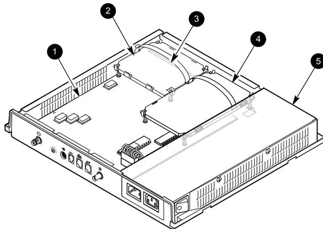
**Install the SIMM cards on the memory controller board.**
