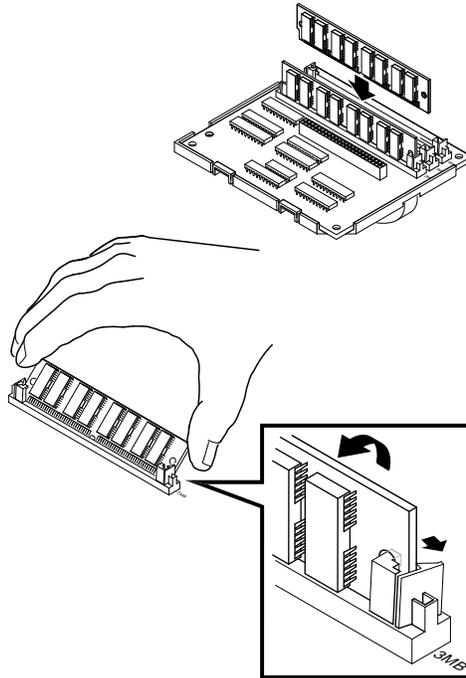
**Install the memory controller board into the system box.**
