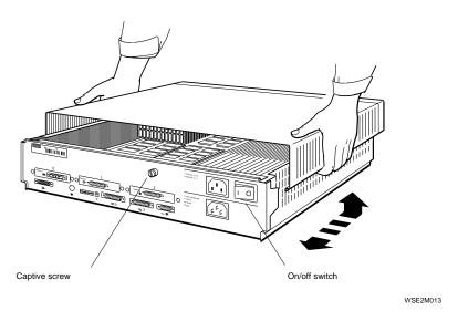
Figure 2-3. Remove and installing the system unit cover
