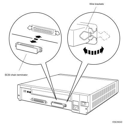
Figure 2-9. Removing and installing a SCSI chain terminator
