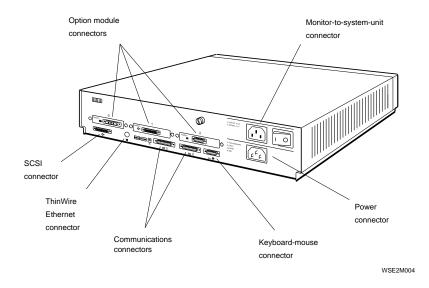
Figure 1-4. DECstation/DECsystem 5000 connectors
