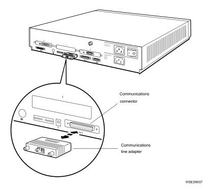
Figure 2-10. Removing and installing a communications line adapter
