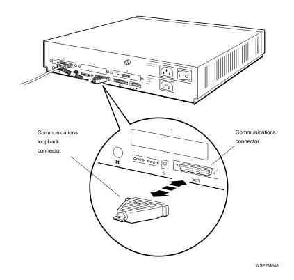
Figure 2-8. Removing and installing a communications loopback connector
