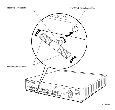
Figure 2-6. Removing and installing a ThinWire Ethernet terminator
