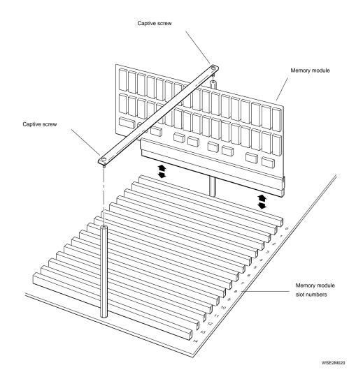
Figure 5-6. Removing and installing a memory module
