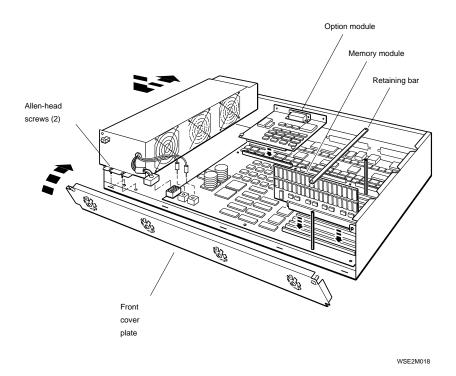
Figure 5-3. Installing hardware on a new system module
