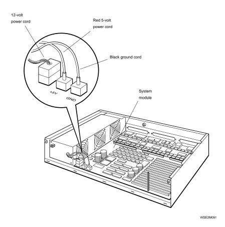
Figure 5-10. System module power cord connections
