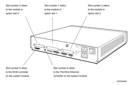
Figure 3-1. Slot numbers for system hardware
