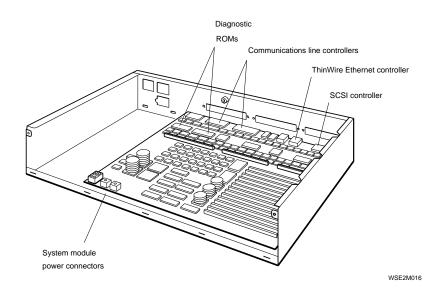
Figure 5-1. System module and chassis
