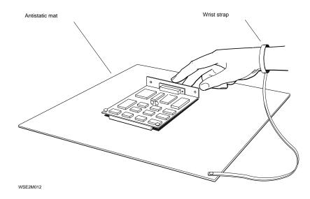
Figure 2-1. Using an antistatic kit
