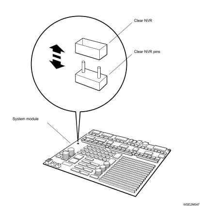
Figure 2-11. Inserting and removing a clear-NVR jumper
