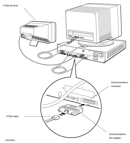
Figure 2-2. Connecting an alternate terminal
