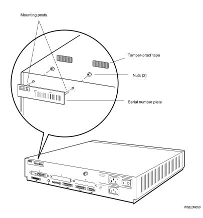
Figure 2-5. Removing and installing a serial number plate
