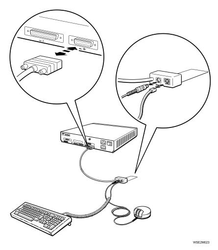
Figure 5-8. Removing and installing a keyboard and mouse
