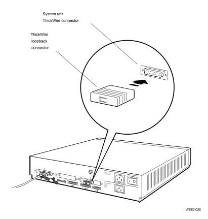
Figure 2-7. Removing and installing a ThickWire loopback connector
