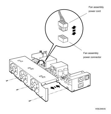
Figure 5-11. Checking the power supply fan assembly connection
