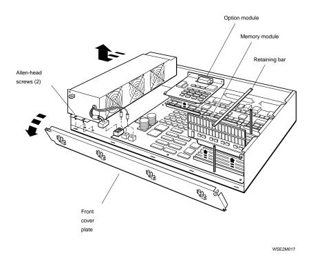
Figure 5-2. Removing hardware from an old system module
