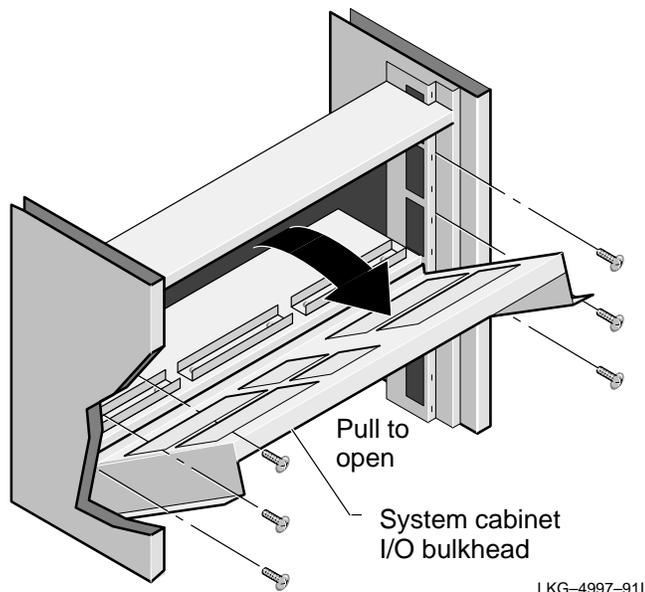
4. Check the cables and cable management bar directly behind the I/O location chosen to install the H3063-A bulkhead. Ensure that any installed cables are fastened under the cable management bar and that the bar is fastened such that it will not contact the H3063-A bulkhead when it is installed.
