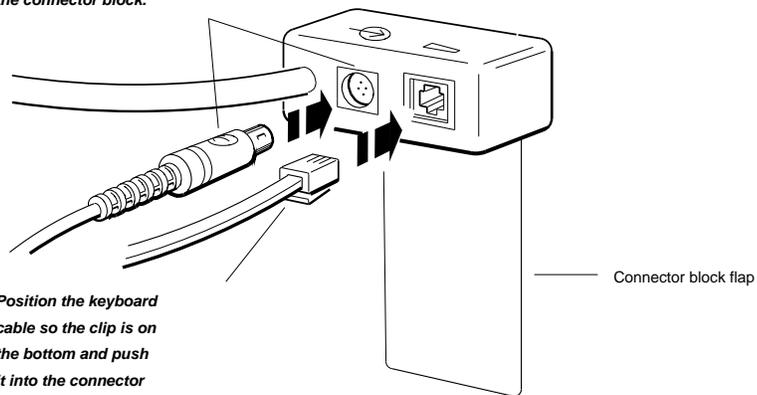
2. *Position the keyboard cable so the clip is on the bottom and push it into the connector block until it clicks into place.*
