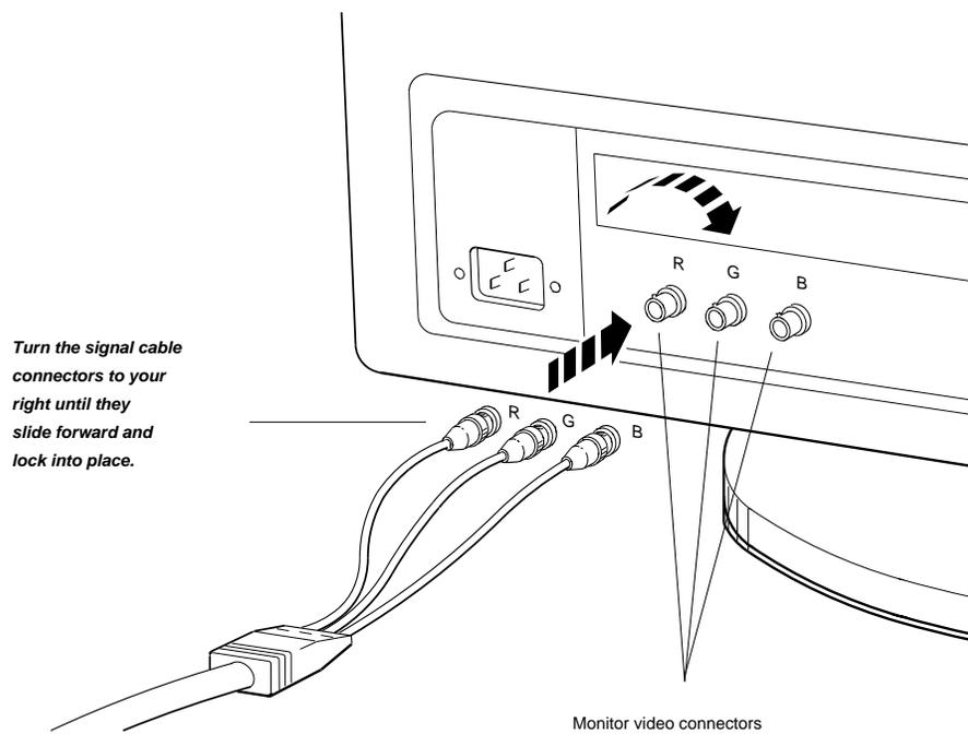
*Turn the signal cable connectors to your right until they slide forward and lock into place.*
