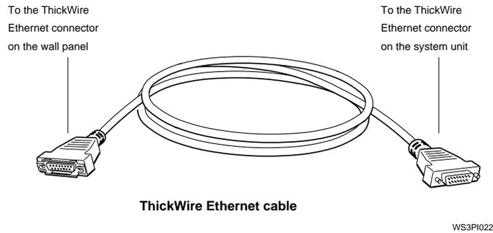
3. Position the cable connector that does *not* have the sliding lock so the widest part is on top. Then push the connector directly onto the base system ThickWire Ethernet connector.
