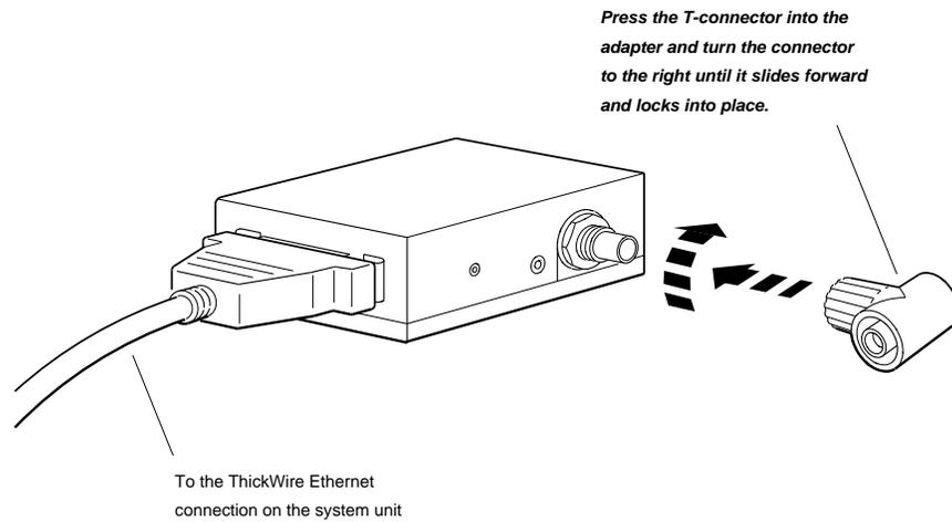
6. If you are connecting the workstation *within* a network cable segment, leave both ends of the T-connector free to attach your in-house network cables.
