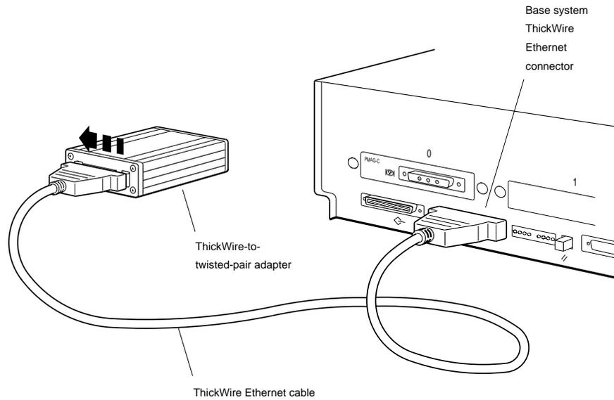
5. Locate the twisted-pair Ethernet cable. Notice that the telephone-jack type of connectors at both ends are identical. Push one of the connectors on the twisted-pair Ethernet cable into the telephone-jack type of connector on the adapter until it clicks into place.
