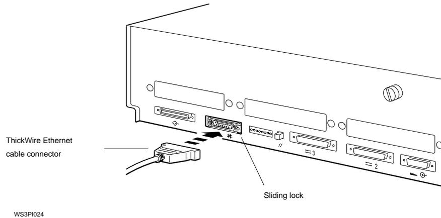
4. To lock the sliding lock on the base system Ethernet connector, push the protruding edge of the lock towards the center of the connector (using a flat-blade screwdriver) until it clicks into place. Check to make sure the cable is locked securely in place before proceeding.
