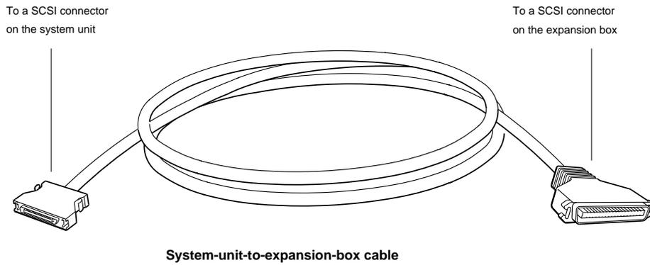
7. Attach the smaller connector on the system-unit-to-expansion-box cable to the SCSI connector on the system unit.
