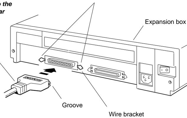
3. Press the two wire brackets firmly against the sides of the cable connector until they click into the grooves on the connector.
