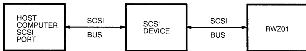
Figure 1-1: Typical System Configuration
