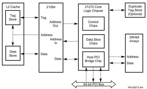
Figure 2–12 Typical Uniprocessor Configuration
