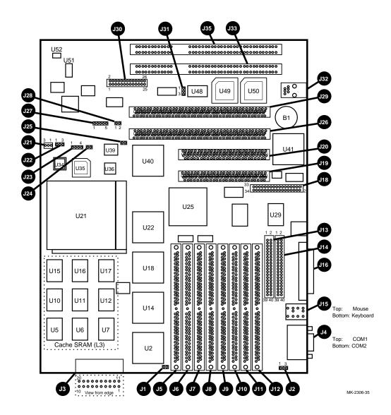
Figure 2–1 AlphaPC 164 Jumper/Connector/Component Location
