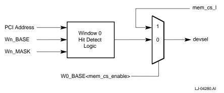
Figure A-22 Memory Chip Select Signal (mem\_cs\_l) Logic
