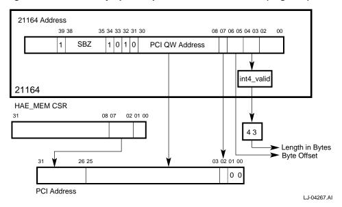
Figure A–9 PCI Memory Sparse Space Address Generation (Region 3)
