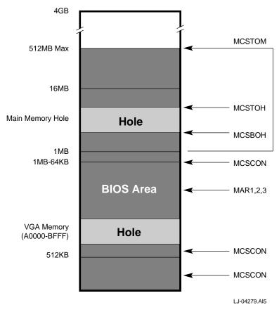
As shown in Figure A–22, PCI window 0 in the CIA can be enabled to accept the **mem\_cs\_l** signal as the PCI memory decode signal. With this path enabled, the PCI window-hit logic simply uses the **mem\_cs\_l** signal. For example, if **mem\_cs\_l** is asserted, then a PCI window 0 hit occurs and the **dev\_sel\_l** signal is asserted on the PCI.
